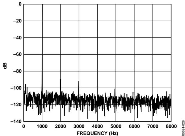
Figure 28. FFT (ADC 16 kHz Direct Sampling)
