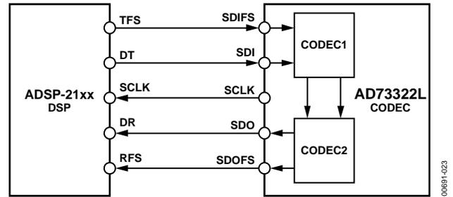
Figure 23. Indirectly Coupled or Nonframe Sync Loop-Back Configuration
