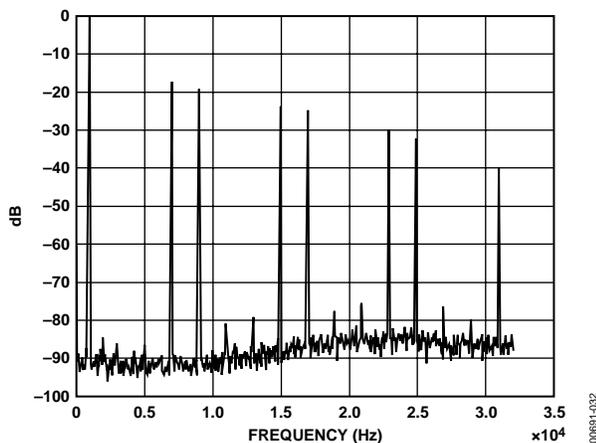
Figure 32. FFT (DAC 8 kHz Sampling—Interpolator Bypassed)
