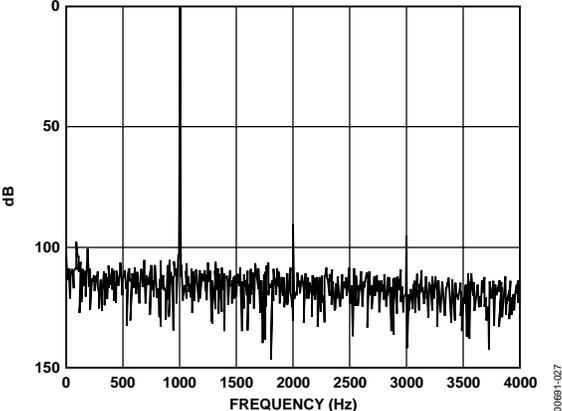
Figure 27. FFT (ADC 8 kHz Direct Sampling)
