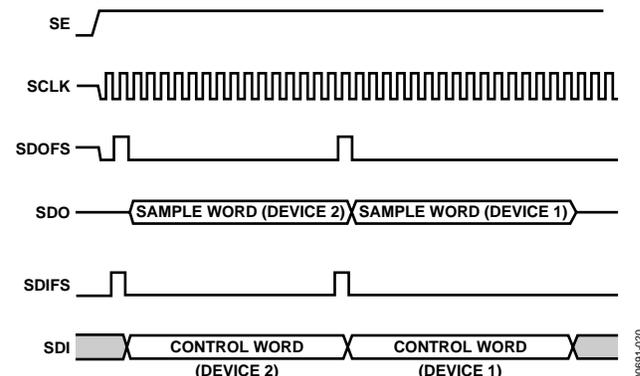
Figure 20. Interface Signal Timing for Control Mode Operation
