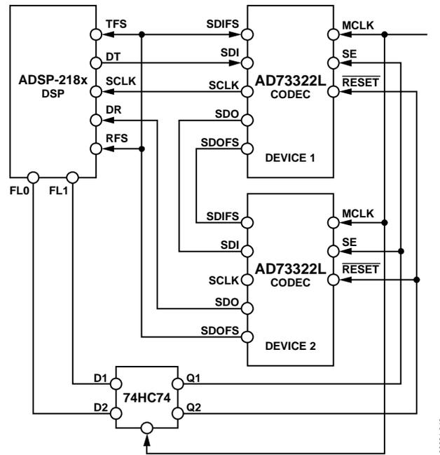
Figure 46. Connection of Two AD73322Ls Cascaded to ADSP-218x
