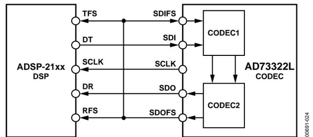
Figure 24. Directly Coupled or Frame Sync Loop-Back Configuration
