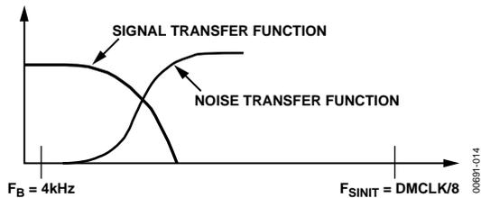
Figure 14. Analog Sigma-Delta Modulator Transfer Function
