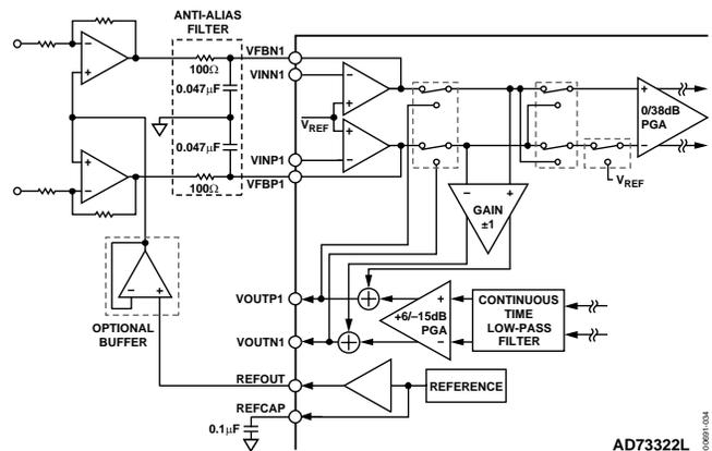
Figure 34. Analog Input (DC-Coupled) Using External Amplifiers
