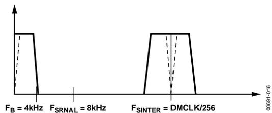
Figure 16. Final Filter (HPF) Transfer Function
