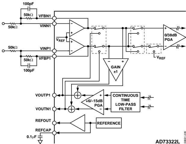
Figure 35. Analog Input (DC Coupled) Using Internal Amplifiers
