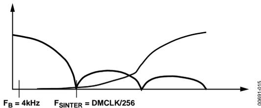
Figure 15. Digital Decimator Transfer Function
