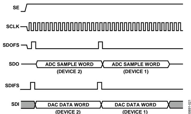
Figure 21. Interface Signal Timing for Data Mode Operation
