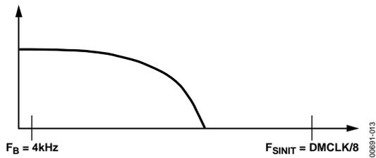
Figure 13. Analog Antialias Filter Transfer Function
