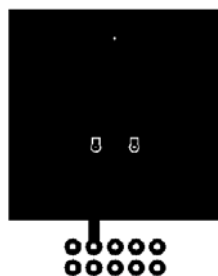
a) 55^\circ\text{C}/\text{W} when mounted on a 1 in 2 pad of 2 oz copper
