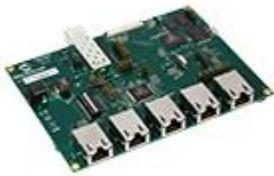
The evaluation board for the KSZ9477S 7-Port Gigabit Ethernet Switch (also KSZ9567 and KSZ8567). The SAMA5D3 processor manages the switch and includes the ATECC508A security encoder. The DSC1101 is the reference clock for GigE communication. The EVB can be used to implement IEEE 1588v2, AVB and DLR/HSR (available on KSZ9477 only) network redundancy. Combine multiple boards to implement redundant networks using free Linux libraries.
