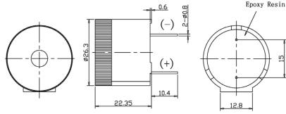
Dimensions : Millimetres Tolerance: ±0.5mm
