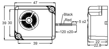
Dimensions : Millimetres Tolerance: ±0.5mm
