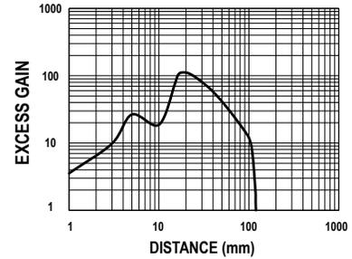
Figure 8. Excess Gain for Standard Sensitivity
