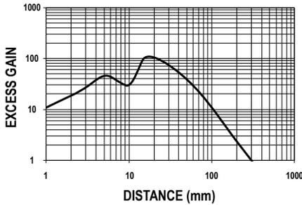
Figure 6. Excess Gain for Standard Sensitivity
