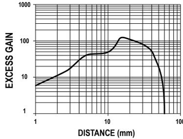
Figure 7. Excess Gain for Standard Sensitivity
