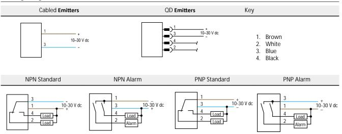
Wiring for the quick disconnect (QD) models is functionally identical.
