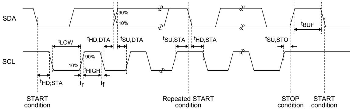
Figure 8. I<sup>2</sup>C Data Timing
