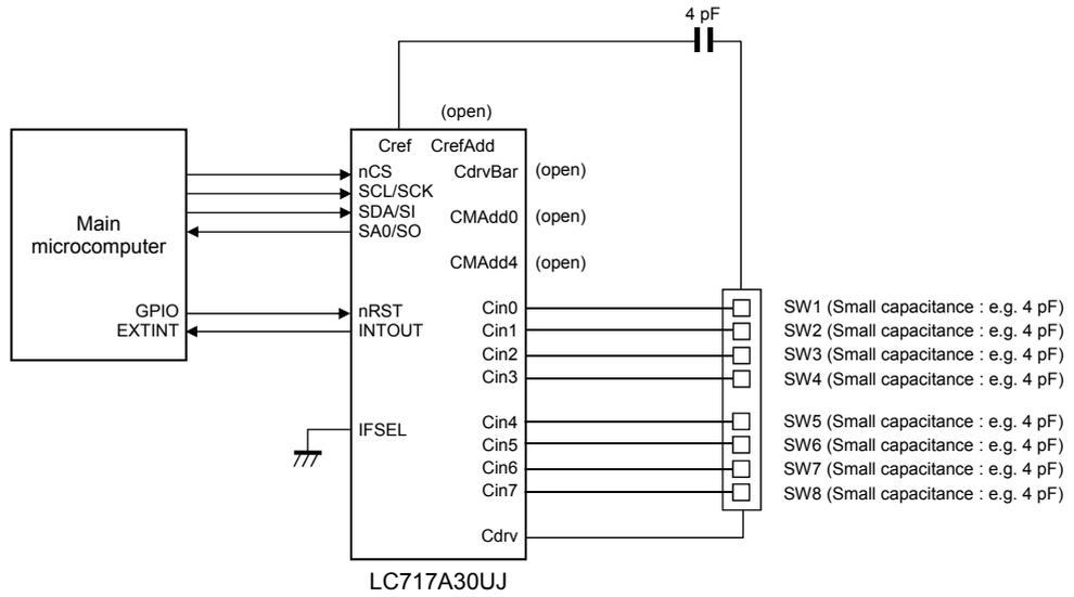
Figure 2. Application Schematic 2
