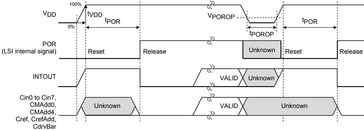
Figure 6. Power-on Sequence by the Power-on Reset
