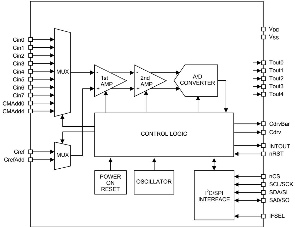
Figure 4. Simplified Block Diagram
