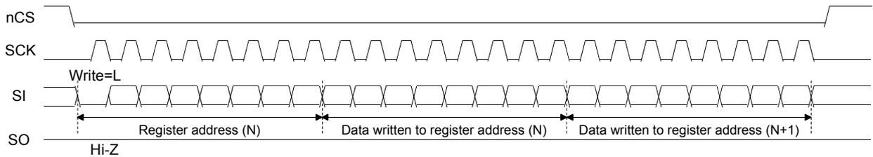
**Figure 12. SPI Write Format**
