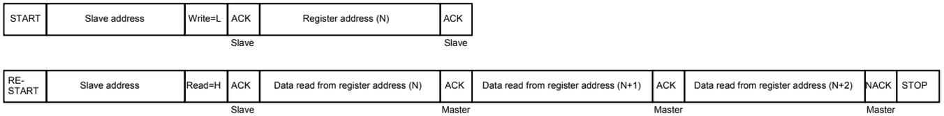
Figure 10. I<sup>2</sup>C Read Format
