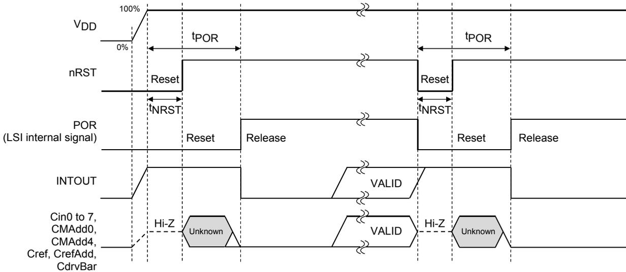
Figure 7. Power-on Sequence by the External Reset
