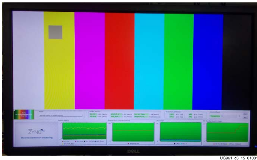
Figure 3-15: HDMI Display for Color Bar Display
