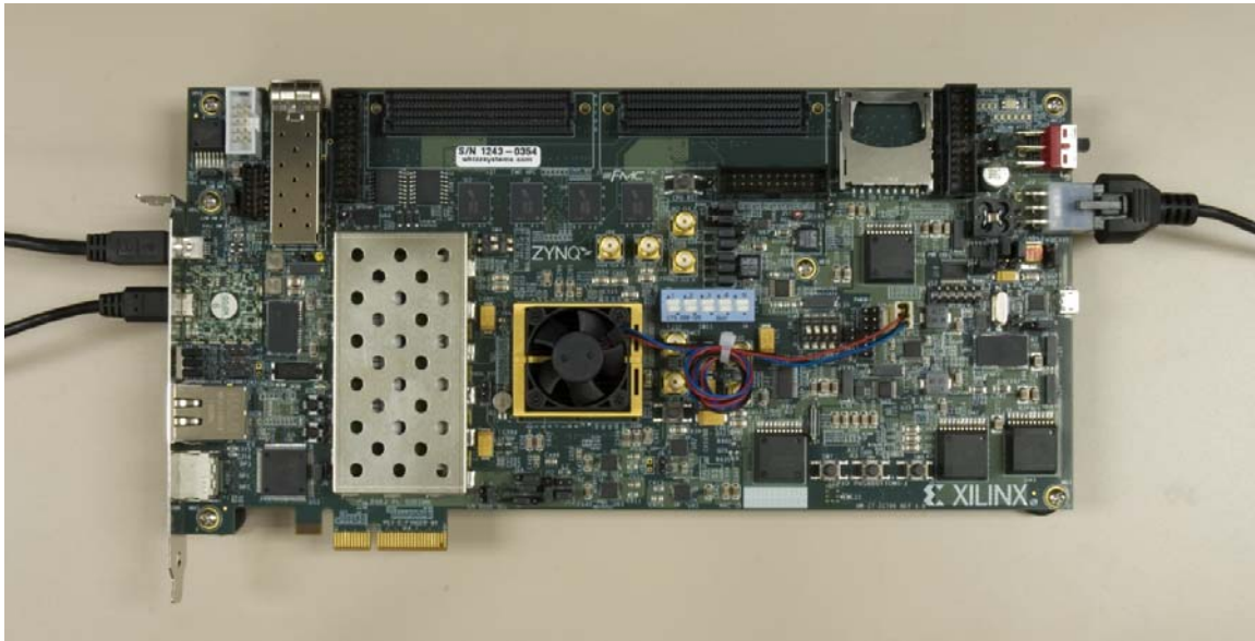
Figure 2-3: ZC706 Board with the UART and Power Cables Attached
