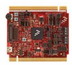
The 32-bit dual-core PXN20 Power Architecture MCU supports a variety of communication protocols, allowing you to design a cost-effective, reliable industrial gateway with cutting-edge performance. A large amount of on-chip flash, on-chip SRAM with error correction code capability, 36-channel ADC, dual cores and a host of serial I/Os make the PXN20 a compelling solution for your next design cycle.
