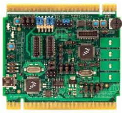
The PXS devices are 32-bit Power Architecture embedded MCUs designed for safety critical applications. All devices in this family are built around a dual core safety architecture and offer more processing power and larger memory sizes to handle a variety of industrial designs. The dual-core can be operated in lockstep mode (redundant processing and calculations) or decoupled parallel mode (independent core operations). The PXS MCUs are SafeAssure solutions.
