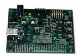
The MC56F802x/3x family combines the processing power of a DSP with the functionality and ease of use of an MCU on a single chip. With a flexible set of peripherals, package and memory options from 16 to 64 KB flash memory, CAN and high-resolution PWM/timers running at up to 96 MHz, the 56F8000 series provides a cost-effective high-performance solution.
