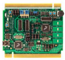
The PXD10 family of 32-bit Power Architecture MCUs provides a cost-effective, single-chip display solution for the industrial market. An integrated TFT driver with digital video input ability from an external video source, significant on-chip memory and low-power design methodologies provide flexibility and reliability in meeting display demands in rugged environments.
