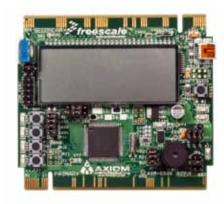
Freescale expands the first S08 ultra-low-power MCU with LCD driver and increased ADC accuracy for medical and metering applications. The MC9S08LH family available with up to 64 KB flash helps you reach your target performance levels while minimizing power consumption in your design, demonstrating extreme energy efficiency for ultra-long operation in battery-powered applications. The S08LH also features a 16-bit ADC for accurate measurement.
