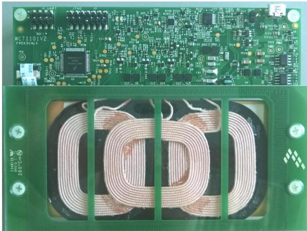
Figure 1 WCT-5WTXMULTI (A28) reference board
