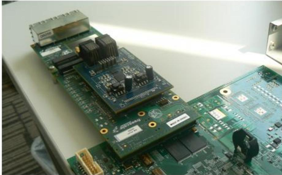
Figure 11 Insert T1/E1 PMC card and Voice card
