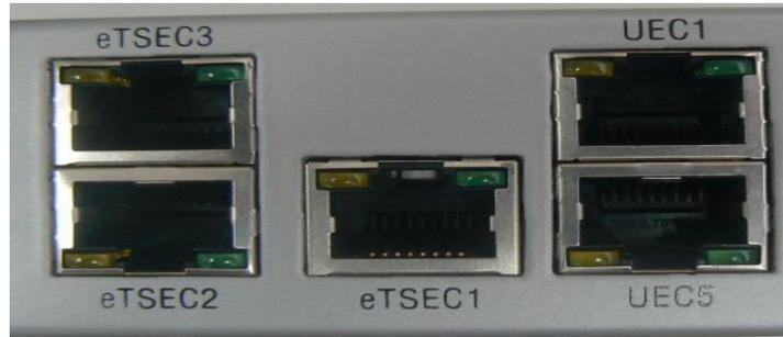
Figure 3: Ethernet Ports on P1025RDB-PA
