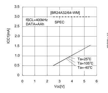
Figure 8. Current consumption at WRITE operation ICC1 (fSCL=400kHz)
