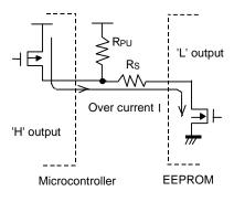
Figure 54. I/O circuit diagram
