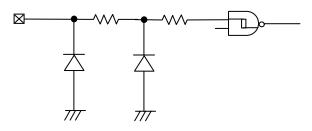
Figure 57. Input pin circuit diagram
