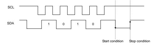
Figure 49. Case of cancel by start, stop condition during slave address input
