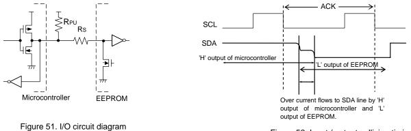
Figure 52. Input / output collision timing
