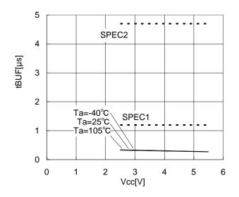
Figure 25. Bus release time before transfer start tBUF
