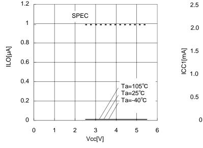
Figure 6. Output leak current ILO(SDA)
