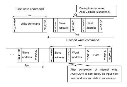
Figure 47. Case to continuously write by acknowledge polling
