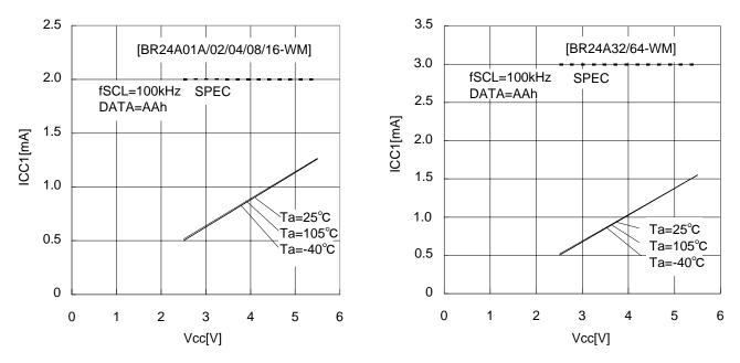
Figure 10. Current consumption at WRITE operation ICC1 (fSCL=100kHz)
