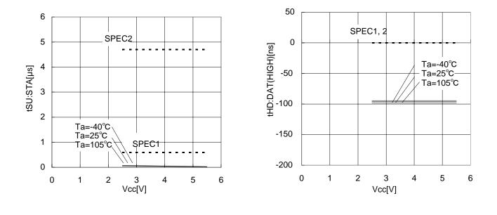
Figure 18. Start condition setup time tSU:STA
