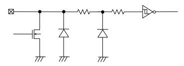
Figure 56. Input / output pin circuit diagram
