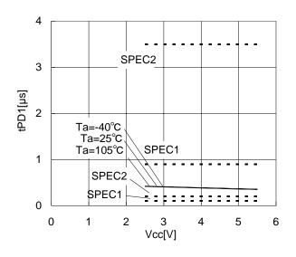
Figure 24. Output data delay time tPD1
