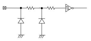
Figure 55. Input pin circuit diagram
