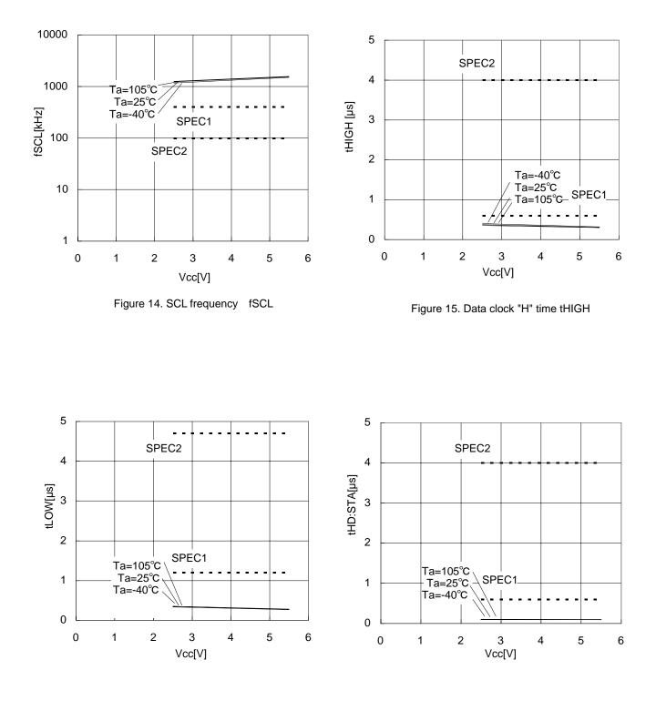
Figure 16. Data clock "L" time tLOW
