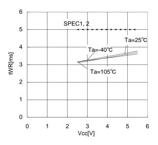
Figure 26. Internal write cycle time tWR
