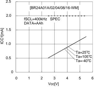
Figure 7. Current consumption at WRITE operation ICC1 (fSCL=400kHz)
