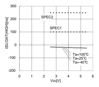
Figure 21. Input data setup time tSU:DAT(HIGH)
