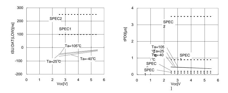
Figure 22. Input data setup time tSU:DAT(LOW)
