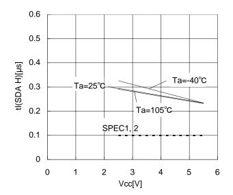
Figure 29. Noise removal valid time tI(SDA H)
