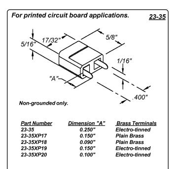
Standard version will be supplied without a mounting hole. 0.097" diameter hole in housing is an option.
