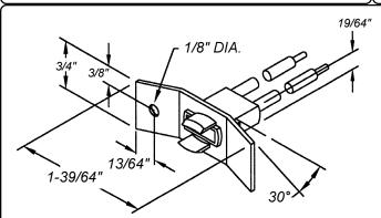
Designed for snap-in mounting with a mechanical locking feature for greater panel assurance.
