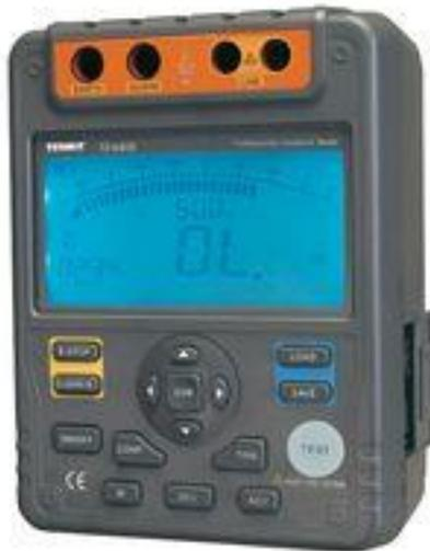
**2500V Digital Insulation Resistance Tester**
