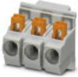
PCB terminal block, Nominal current: 24 A, Nom. voltage: 630 V, Pitch: 7.5 mm, Number of positions: 3, Connection method: Push-in spring connection, Mounting: Wave soldering, Article with lateral pin exit
