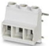
PCB terminal block, Nominal current: 24 A, Nom. voltage: 630 V, Pitch: 7.5 mm, Number of positions: 3, Connection method: Screw connection with tension sleeve, Mounting: Wave soldering, Article with lateral pin exit
