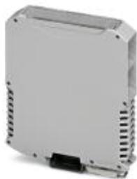
Complete housing with vents, Complete housing, Cross connection: DIN rail bus connector, Color: light gray, Width: 22.5 mm, Constructional height: 114.5 mm, Number of positions cross connector: 5
