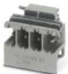
Header, Nominal current: 16 A, Rated voltage (III/2): 320 V, Number of positions: 4, Pitch: 5 mm, Color: light gray, Mounting: Soldering
