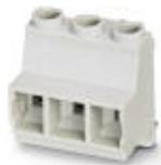
PCB terminal block, Nominal current: 24 A, Nom. voltage: 630 V, Pitch: 7.5 mm, Number of positions: 3, Connection method: Screw connection with tension sleeve, Mounting: Wave soldering, Article with lateral pin exit
