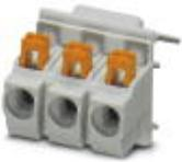
PCB terminal block, Nominal current: 24 A, Nom. voltage: 630 V, Pitch: 7.5 mm, Number of positions: 3, Connection method: Push-in spring connection, Mounting: Wave soldering, Article with lateral pin exit
