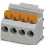
PCB terminal block, Nominal current: 22 A, Nom. voltage: 250 V, Pitch: 5 mm, Number of positions: 4, Connection method: Push-in spring connection, Mounting: Wave soldering, Conductor/PCB connection direction: 0 °, Color: light gray, Article with lateral pin exit
