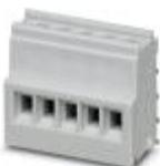
PCB terminal block, Nominal current: 8 A, Nom. voltage: 160 V, Pitch: 3.5 mm, Number of positions: 5, Connection method: Screw connection with tension sleeve, Mounting: Wave soldering, Conductor/PCB connection direction: 0 °, Article with lateral pin exit
