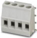
PCB terminal block, Nominal current: 24 A, Nom. voltage: 320 V, Pitch: 5 mm, Number of positions: 4, Connection method: Screw connection with tension sleeve, Mounting: Wave soldering, Conductor/PCB connection direction: 0 °, Article with lateral pin exit
