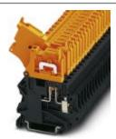
Disconnect terminal block, Connection type: Screw connection, Cross section: 0.14 mm² - 6 mm², AWG: 26 - 10, Nominal current: 20 A, Nominal voltage: 500 V, Length: 57.8 mm, Width: 6.2 mm, Color: black/orange, Assembly: NS 35/7,5, NS 35/15
