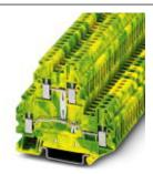
Protective conductor double-level terminal block, Connection type: Screw connection, Cross section: 0.14 mm² - 4 mm², AWG: 26 - 12, Width: 5.2 mm, Color: green-yellow, Mounting type: NS 35/7,5, NS 35/15
