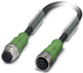
Sensor/Actuator cable, 8-position, PUR halogen-free, black-gray RAL 7021, Plug straight M12, A-coded, on Socket straight M12, A-coded, Cable length: 3 m
