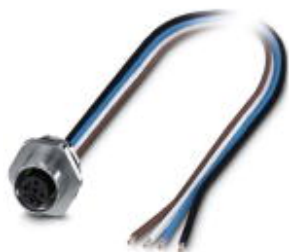
Flush-type connector, Universal, 5-position, SocketLink:M12, A-coded, Front mounting, M16 x 1.5, Individual wires, Cable length: 0.5 m
