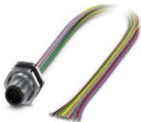
Flush-type connector, Universal, 17-position, PlugLink:M12, A-coded, Rear mounting, M16 x 1.5, Individual wires, Cable length: 0.5 m
