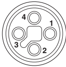
Pin assignment of M12 socket, 4-pos., T-coded, socket side view
