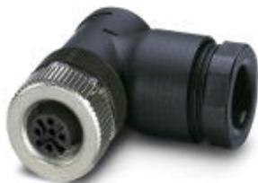
Power connectors, 5-position, Socket angled M12, A-coded, Screw connection, Knurl material: Zinc die-cast, nickel-plated, Cable gland Pg11, External cable diameter 8 mm ... 10 mm
