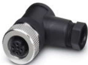
Sensor/actuator connector, female, angled, 5-pos., M12, A-coded, screw connection, metal knurl, cable screw connection Pg7
