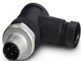
Connector, 4-position, Plug angled M12, A-coded, Screw connection, Knurl material: Zinc die-cast, nickel-plated, Cable gland Pg7, External cable diameter 4 mm ... 6 mm
