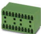
Header, Nominal current: 8 A, Rated voltage (III/2): 160 V, Number of positions: 10, Pitch: 3.81 mm, Color: green, Contact surface: Tin, Mounting: Wave soldering, In combination with MCV plug components, both an MCVW and an MCVR plug must be used.
