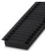
Header, Nominal current: 8 A, Rated voltage (III/2): 160 V, Number of positions: 10, Pitch: 3.81 mm, Color: black, Contact surface: Tin, Mounting: THR soldering, User information and design recommendations for through hole reflow technology can be found under "Downloads"
