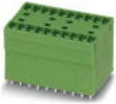
Header, Nominal current: 8 A, Rated voltage (III/2): 160 V, Number of positions: 10, Pitch: 3.81 mm, Color: green, Contact surface: Tin, Mounting: Wave soldering, In combination with MCV plug components, both an MCVW and an MCVR plug must be used.
