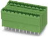
Header, Nominal current: 10 A, Rated voltage (III/2): 320 V, Number of positions: 10, Pitch: 5.08 mm, Color: green, Contact surface: Tin, Mounting: Wave soldering, In combination with MVSTB or FKCV plug components, both an MVSTBW (or FKCVW) and an MVSTBR plug (or FKCVR) must be used. Combination with TMSTBP plug components is not possible!
