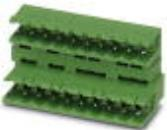
Header, Nominal current: 10 A, Rated voltage (III/2): 320 V, Number of positions: 10, Pitch: 5.08 mm, Color: green, Contact surface: Tin, Mounting: Wave soldering, Can be aligned! Mounting flange: Order No. 1736771, 1736768. In combination with MVSTB or FKCV plug components, both an MVSTBW (or FKCVW) and an MVSTBR plug (or FKCVR) must be used. Combination with TMSTBP plug components is not possible!
