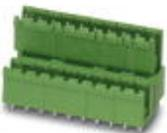
Header, Nominal current: 10 A, Rated voltage (III/2): 320 V, Number of positions: 10, Pitch: 5.08 mm, Color: green, Contact surface: Tin, Mounting: Wave soldering, Can be aligned! Mounting flange: Order No. 1836477, 1836480. In combination with MVSTB or FKCV plug components, both an MVSTBW (or FKCVW) and an MVSTBR plug (or FKCVR) must be used. Combination with TMSTBP plug components is not possible!
