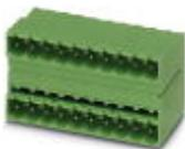
Header, Nominal current: 10 A, Rated voltage (III/2): 320 V, Number of positions: 9, Pitch: 5.08 mm, Color: green, Contact surface: Tin, Mounting: Wave soldering, In combination with MVSTB or FKCV plug components, both an MVSTBW (or FKCVW) and an MVSTBR plug (or FKCVR) must be used. Combination with TMSTBP plug components is not possible!
