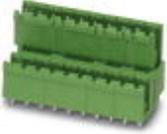
Header, Nominal current: 10 A, Rated voltage (III/2): 320 V, Number of positions: 9, Pitch: 5.08 mm, Color: green, Contact surface: Tin, Mounting: Wave soldering, Can be aligned! Mounting flange: Order No. 1836477, 1836480. In combination with MVSTB or FKCV plug components, both an MVSTBW (or FKCVW) and an MVSTBR plug (or FKCVR) must be used. Combination with TMSTBP plug components is not possible!
