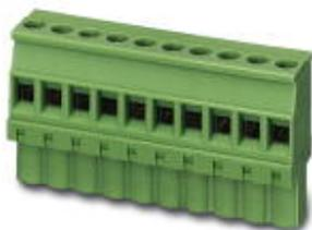
Plug component, Nominal current: 12 A, Rated voltage (III/2): 320 V, Number of positions: 9, Pitch: 5.08 mm, Connection method: Screw connection with tension sleeve, Color: green, Contact surface: Tin
