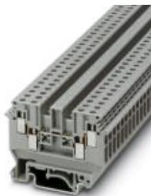
1-level terminal block with double connection on both sides, cross section: 0.2 - 2.5 mm<sup>2</sup>, AWG: 30 - 10, width: 6.2 mm, color: Gray
