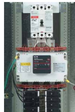
The SPD Series is also available as an integrated unit interfaced via a circuit breaker unit resident in the electrical assembly. This installation keeps connected lead lengths short while providing a means of disconnecting power to the unit quickly and easily.
