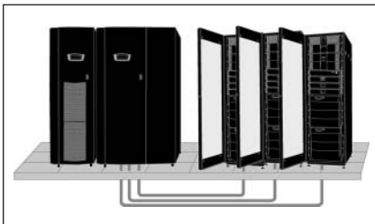
Figure 33.2-28. Typical Application of Eaton 9390 Integrated Distribution Cabinet Distributing Power to IT Racks
