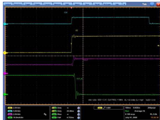
Figure 17: Turn OFF output current characteristics (2)
