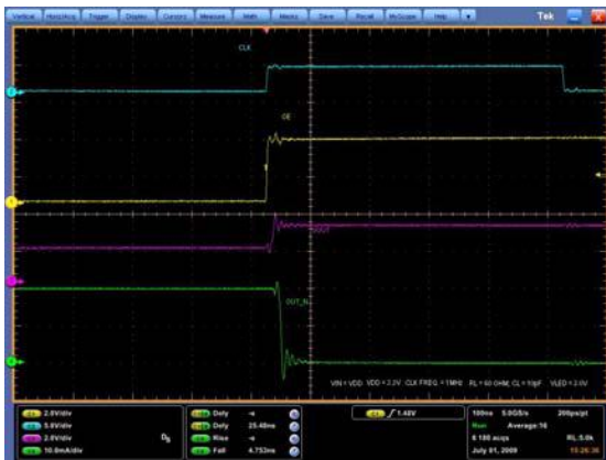
Figure 16: Turn ON output current characteristics (1)
