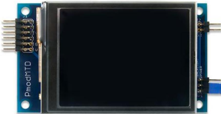
The Digilent Pmod MTDS (Revision A) is a gorgeous 2.8" touchscreen display with a powerful on-board microcontroller that performs graphics processing tasks. The display is a capacitive touchscreen with QVGA resolution (320x240) and 2 finger multi-touch support.
