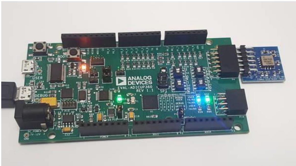
The application reads the **X**, **Y**, and **Z** acceleration registers. The acceleration in the 3 axis is displayed in [**G**]. There is an internal temperature sensor in the ADXL355, which is converted by the on chip 12-bit ADC. The acceleration range can also be selected by setting the **ADXL355\_RANGE** variable with the `ADXL355.h` file. (Values of [2, 4, and 8 are acceptable] )
