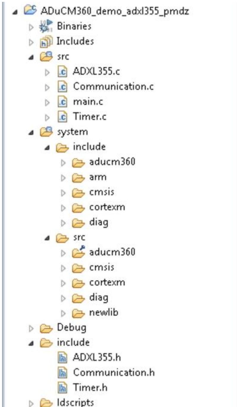
In the **src** and **include** folders you will find the source and header files related to ADXL355 application. You can modify as you wanted those files. The *Communication.c/h* files contain SPI and UART specific data, meanwhile the *ADXL355.c/h* files contain the accelerometer data. Here are parameters you can configure:
