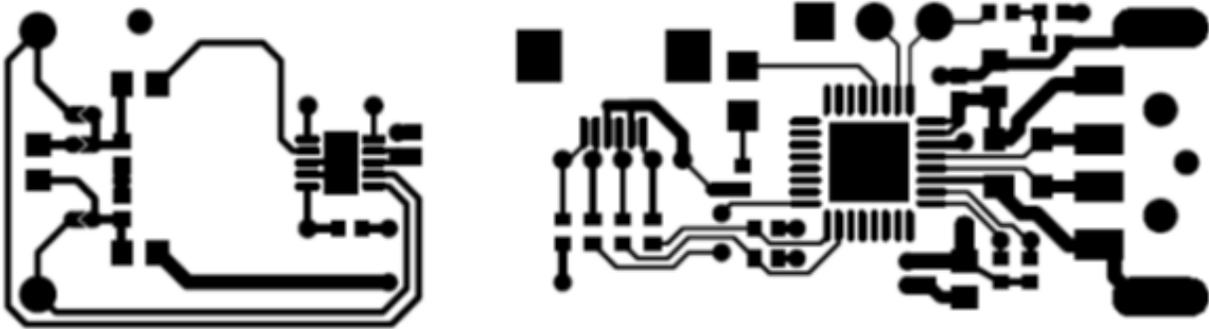
Figure 13. Si7013 Dongle Board Layout Top Layer
