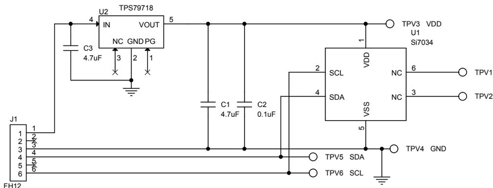
Figure 19. Si7034 Schematic
