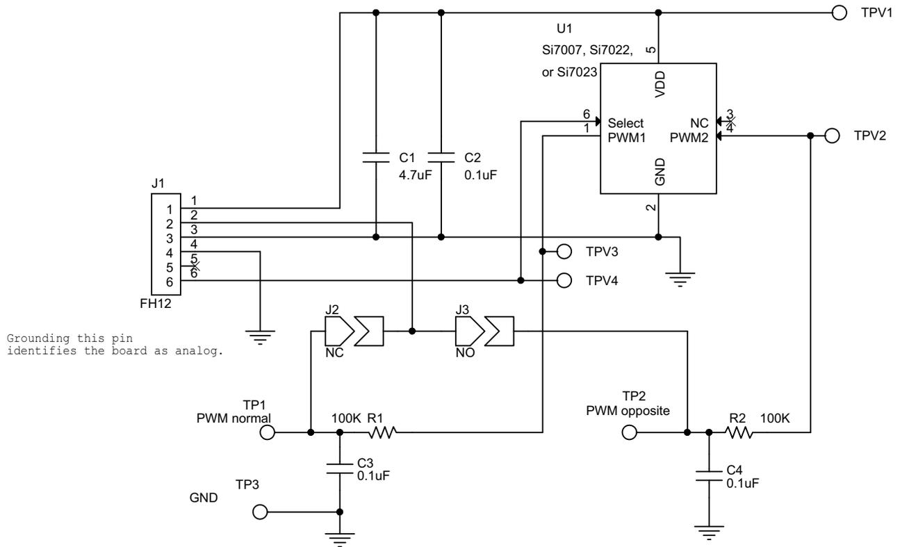
Figure 18. Si7007, Si7022, and Si7023 EVB Schematic
