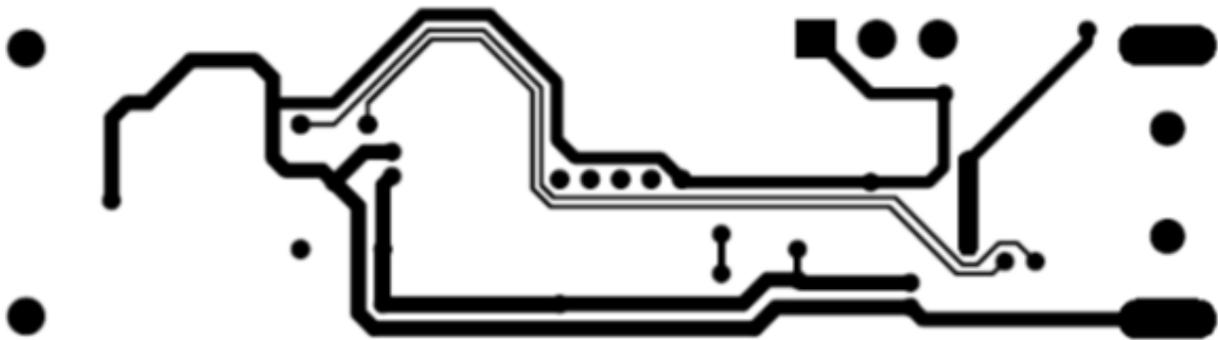
Figure 14. Si7013 Dongle Board Layout Bottom Layer
