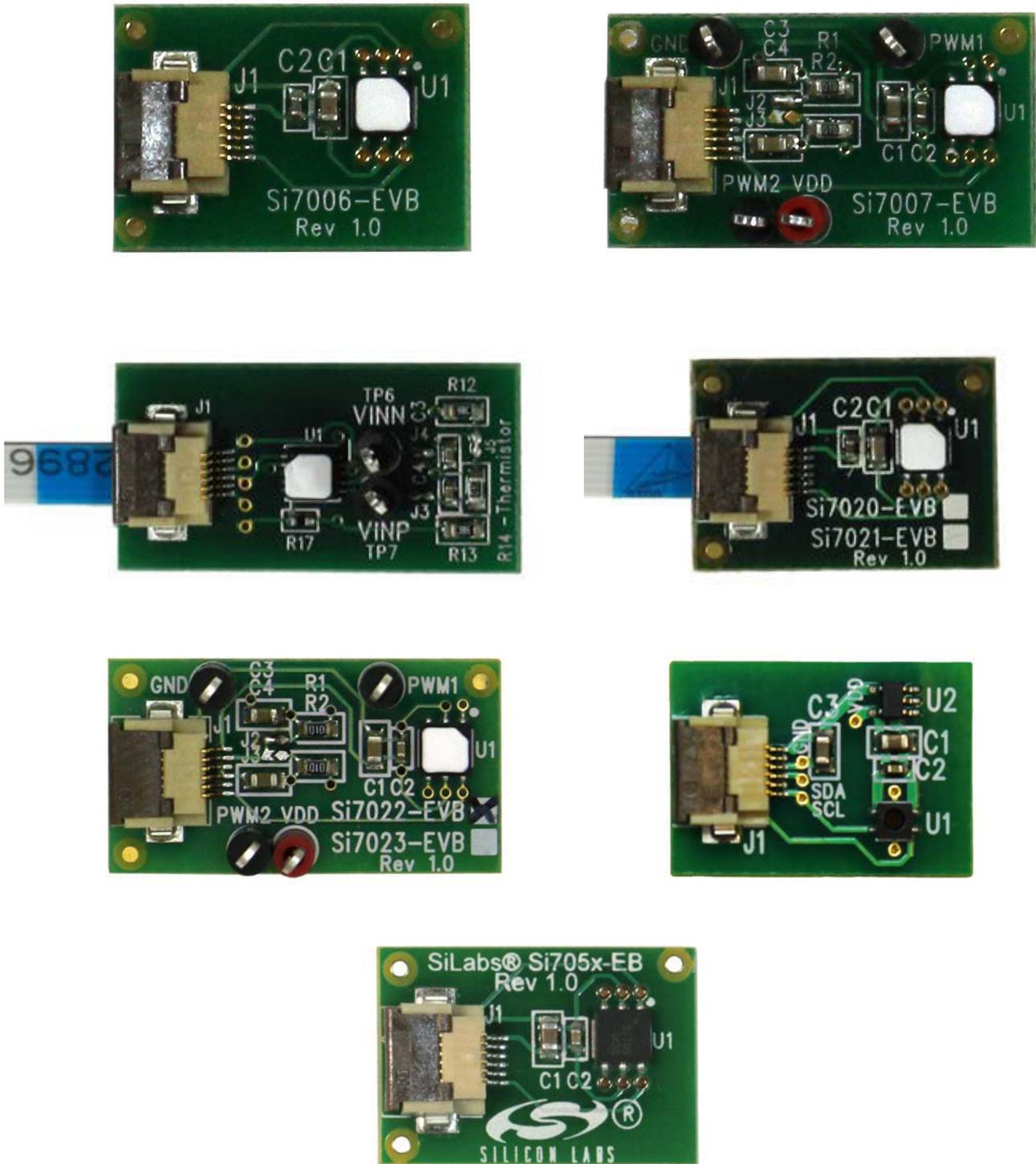
Figure 2. Si7006, Si7007, Si7013, Si7020/21, Si7022/23, Si7034/Si7057, and Si705x Evaluation Boards
