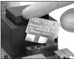
This unique voltage selector PCB displays the operating voltage selected. To change the voltage, disconnect power to the meter. Remove the selector, reverse the selector and fully re-insert it in the socket. This selector is not required for optional power supplies.
