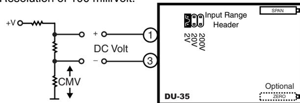
Max CMV (common mode voltage) is 50V.\*
