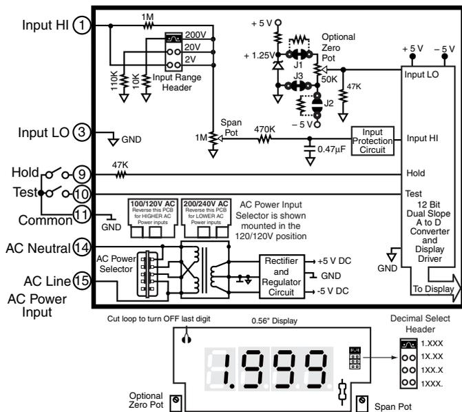
**Pins 14 & 15 - AC Power Input:** These pins are the Power Input pins for the meter. All DU-Series meters sold in North America are pre-configured at the factory for 100/120V AC operation. To re-configure for 200/240V AC operation, simply pull out the AC Power Voltage Selector located directly behind the transformer, turn it around and re-insert it into the socket so that "200/240V AC" is visible. Various other AC/DC power options are available. See Ordering Information for details.
