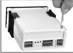
To open back panel, insert a flat screwdriver or similar instrument in both slots on the top of the case and pry open. The DU-Series meters slide out from the rear of the case as a complete assembly.
