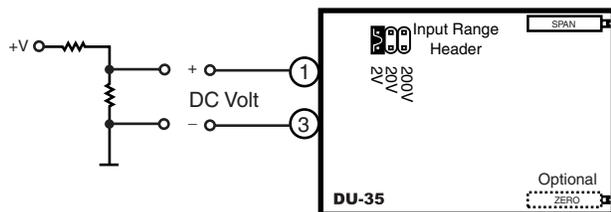
**DC Volts Differential** measurement with a Resolution of 100 milliVolt.
