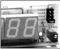
Decimal selection is made on the front of the display board by moving the jumper to the indicated position on the header for the decimal required.
