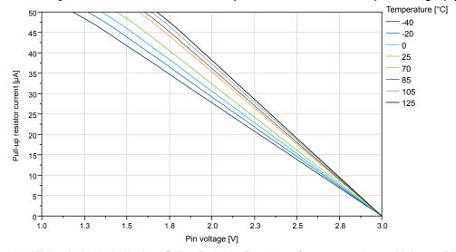
Figure 38-30. ATtiny1614/1616/1617: IO Pin Pull-Up Resistor Current vs. Input Voltage (V<sub>DD</sub>=5.0V)
