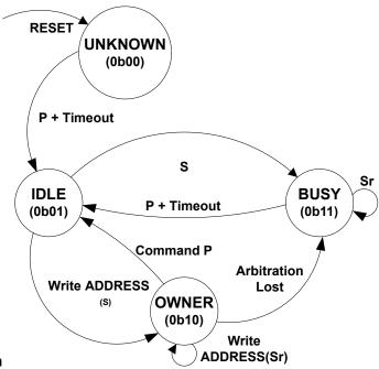
Figure 26-12. Bus State, State Diagram
