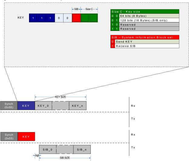
The Figure above shows the transmission of a KEY, and the reception of a SIB. In both cases, the  $SIZE\_C$  field in the opcode determines the number of frames to be sent or received. There is no response after sending a KEY to the UPDI. When requesting the SIB, data will be transmitted from the UPDI according to the current Guard Time setting.
