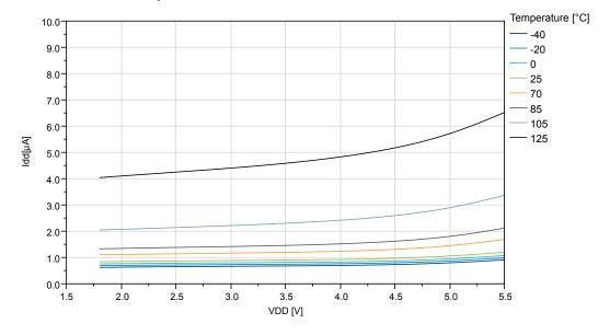
Figure 38-13. ATtiny1614/1616/1617: Standby Mode Supply Current vs.  $V_{DD}$  (RTC running with internal OSCULP32K)
