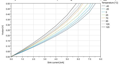
Figure 38-21. ATtiny1614/1616/1617: IO Pin Output Voltage vs. Sink Current (V<sub>DD</sub>=3.0V)
