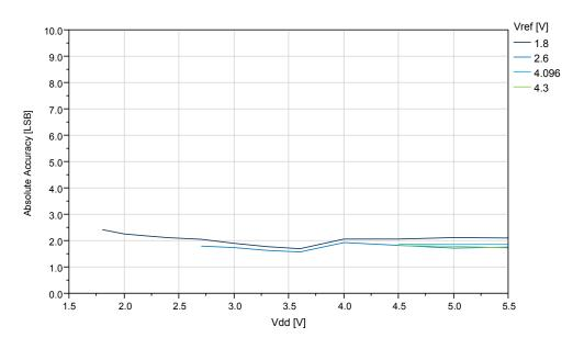
Figure 38-52. ATtiny1614/1616/1617 REFSEL = External reference, Absolute Accuracy vs.  $V_{REF}$  ( $V_{DD}$ =5.0V,  $f_{ADC}$ =115ksps)
