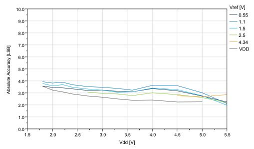
Figure 38-42. ATtiny1614/1616/1617: REFSEL = Internal reference, Absolute Accuracy vs. V<sub>REF</sub> (V<sub>DD</sub>=5.0V, f<sub>ADC</sub>=115ksps)
