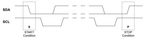
Multiple START conditions can be issued during a single transaction. A START condition that is not directly following a STOP condition is called a repeated START condition (Sr).
