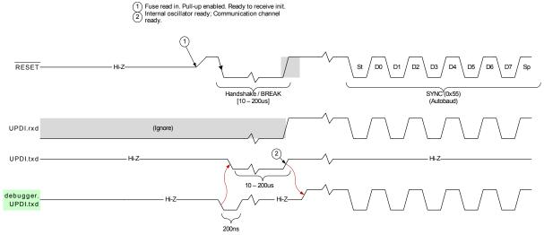
When the pull-up is detected, the debugger initiates the enable sequence by driving the line low for a minimum of 200ns and a maximum of 1us to ensure that the line is released from the debugger before the UPDI enable sequence is done.
