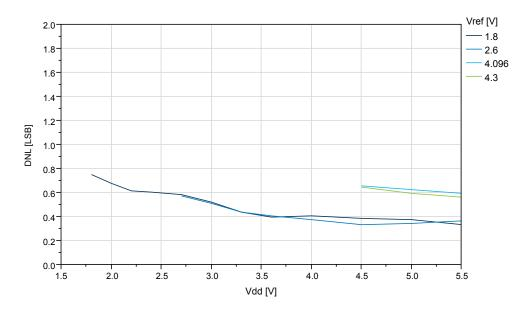
Figure 38-54. ATtiny1614/1616/1617 REFSEL = External reference, DNL vs.  $V_{REF}$  ( $V_{DD}$ =5.0V,  $f_{ADC}$ =115ksps)
