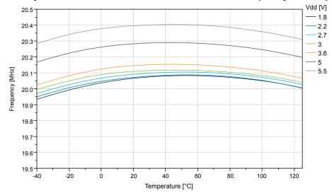
Figure 38-68. ATtiny1614/1616/1617: OSC20M Internal Oscillator: Frequency vs. V<sub>DD</sub>
