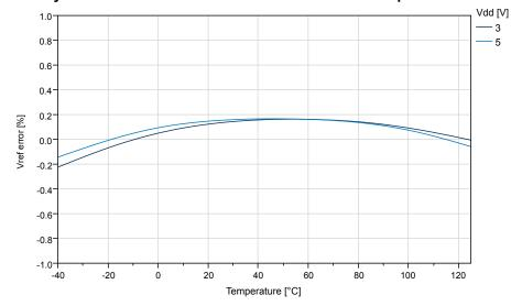
Figure 38-34. ATtiny1614/1616/1617: Internal 4.34V Reference vs. Temperature
