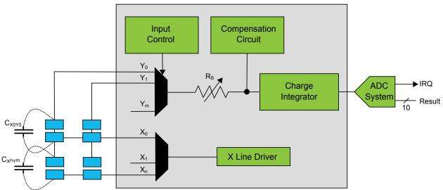
Figure 32-2. PTC Block Diagram Self-Capacitance
