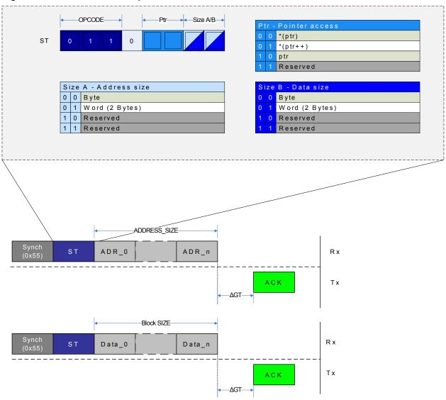
The Figure above gives an example of ST to the UPDI pointer register, and store of regular data. In both cases an Acknowledge (ACK) is sent back by the UPDI if the store was successful, and a SYNCH character is sent before each instruction. To write the UPDI pointer register, the following procedure should be followed.
