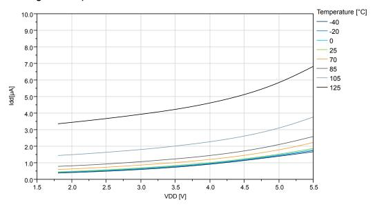
Figure 38-15. ATtiny1614/1616/1617: Standby Mode Supply Current vs. V<sub>DD</sub> (Sampled BOD running at 1kHz)
