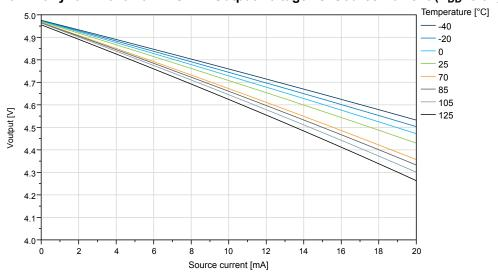
Figure 38-27. ATtiny1614/1616/1617: IO Pin Output Voltage vs. Source Current (T=25°C)
