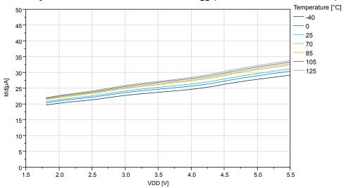
Figure 38-36. ATtiny1614/1616/1617: BOD Current vs. V<sub>DD</sub> (Sampled BOD at 125Hz)
