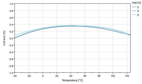
Figure 38-32. ATtiny1614/1616/1617: Internal 1.1V Reference vs. Temperature
