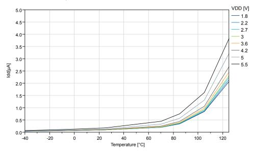
Figure 38-11. ATtiny1614/1616/1617: Power Down Mode Supply Current vs.  $V_{\rm DD}$  (all functions disabled)
