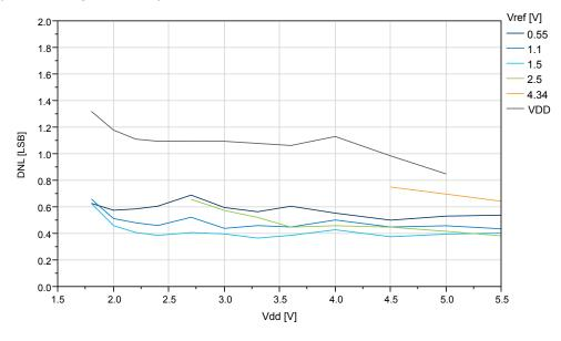
Figure 38-44. ATtiny1614/1616/1617: REFSEL = Internal reference, DNL vs.  $V_{REF}$  ( $V_{DD}$ =5.0V, f<sub>ADC</sub>=115ksps)
