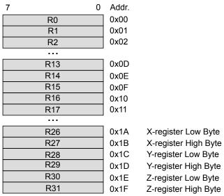
The register file is located in a separate address space and is therefore not accessible trough instructions operation on data memory.
