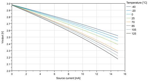
Figure 38-26. ATtiny1614/1616/1617: IO Pin Output Voltage vs. Source Current (V<sub>DD</sub>=5.0V)
