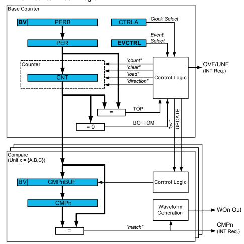
Figure 20-2. Timer/Counter Block Diagram
