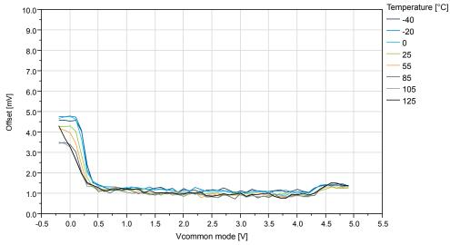
Figure 38-64. ATtiny1614/1616/1617: Offset vs.  $V_{CM}$  - 10mV to 50mV ( $V_{DD}$ =5V, T=25°C)
