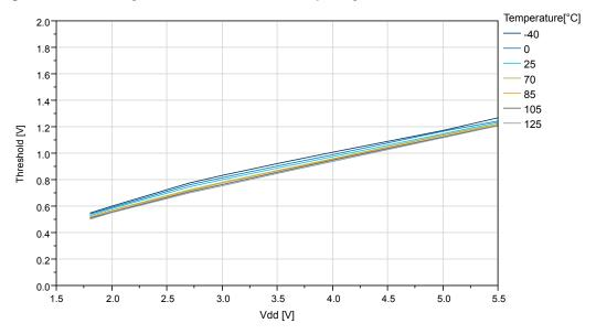
Figure 38-17. ATtiny1614/1616/1617: IO Pin Input Threshold Voltage vs. V<sub>DD</sub> (T=25°C)
