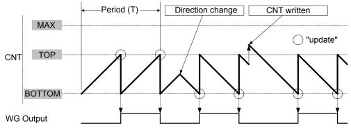
The waveform frequency ( $f_{FRO}$ ) is defined by the following equation:
