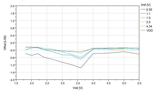
Figure 38-50. ATtiny1614/1616/1617: REFSEL = Internal reference, Offset Error vs.  $V_{REF}$  ( $V_{DD}$ =5.0V,  $f_{ADC}$ =115ksps)
