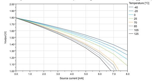
Figure 38-25. ATtiny1614/1616/1617: IO Pin Output Voltage vs. Source Current (V<sub>DD</sub>=3.0V)
