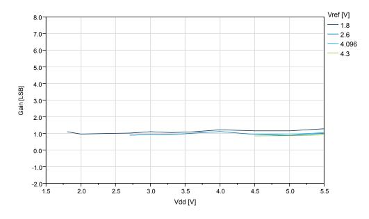
Figure 38-56. ATtiny1614/1616/1617 REFSEL = External reference, Gain vs.  $V_{REF}$  ( $V_{DD}$ =5.0V,  $f_{ADC}$ =115ksps)
