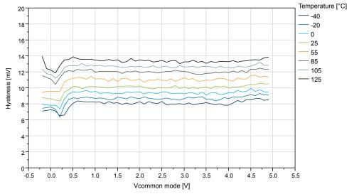
Figure 38-62. ATtiny1614/1616/1617: Hysteresis vs.  $V_{CM}$  - 10mV to 50mV ( $V_{DD}$ =5V, T=25°C)
