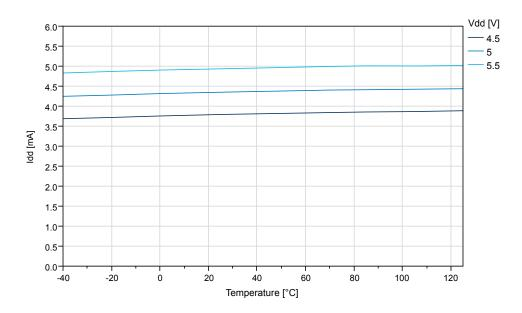
Figure 38-9. ATtiny1614/1616/1617: Idle Supply Current vs. V<sub>DD</sub> (f=32KHz OSCULP32K)
