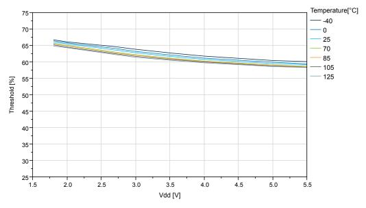
Figure 38-19. ATtiny1614/1616/1617: IO Pin Input Threshold Voltage vs.  $V_{DD} (V_{IL})$
