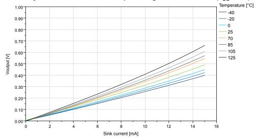
Figure 38-22. ATtiny1614/1616/1617: IO Pin Output Voltage vs. Sink Current (V<sub>DD</sub>=5.0V)
