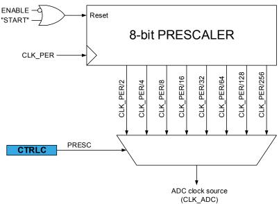
The ADC requires an input clock frequency between 50kHz and 2MHz for maximum resolution. If a lower resolution than 10 bits is selected, the input clock frequency to the ADC can be higher than 2MHz to get a higher sample rate.
