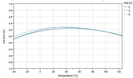
Figure 38-33. ATtiny1614/1616/1617: Internal 2.5V Reference vs. Temperature
