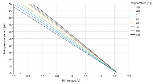
Figure 38-29. ATtiny1614/1616/1617: IO Pin Pull-Up Resistor Current vs. Input Voltage (V<sub>DD</sub>=3.0V)
