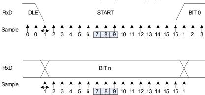
The transmission Baud Rate must be set up in relation to the selected UPDI clock, which can be adjusted by UPDICLKSEL in UPDI.ASI\_CTRLA. See Table 33-2 for recommended maximum and minimum baud rate settings.
