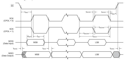
Figure 37-6. SPI - Timing Requirements in Slave Mode
