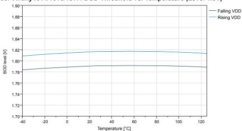
Figure 38-39. ATtiny1614/1616/1617: BOD Threshold vs. Temperature (Level 2.6V)
