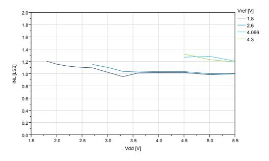
Figure 38-58. ATtiny1614/1616/1617 REFSEL = External reference, INL vs.  $V_{REF}$  ( $V_{DD}$ =5.0V,  $f_{ADC}$ =115ksps)
