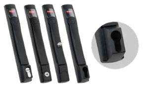
Flush Handles are optional for any solid, window or disconnect door greater than 600mm in height, except Voice/Data and Colocation cabinets. They are ergonomically designed to provide style and function in a low profile. The handle is die-cast zinc finished with RAL 9005 textured black polyester powder paint. Provision to add your logo is included. Handle can be installed to rotate either clockwise or counterclockwise.
