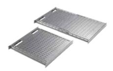
An easy-to-install tool-less vented 19-in. shelf. Mounts onto rack angles that have EIA-spaced square holes (.375 in.). Shelf slides open and provides a variable-sized, continuous surface for equipment. Back of shelf has oval cutouts for power and data cables. Accessory hole patterns at back of shelf fit small and large D-rings to help manage cable. Made of steel with a 150 lb. (68 kg) static load rating. Available with RAL 9005 black or RAL 7035 gray polyester powder coat finish.
