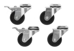
A set of four casters (two locking, two non-locking) that mount directly to the bottom of a PROLINE frame, 0-mm or 100-mm Solid Base or a Console. **(Do not use on plinth bases.)** Casters elevate the enclosure 110 mm (4.33) when installed. Caster frames are plated steel with ball-bearing pivots. Caster wheels are made of a black polyamide material. Kit includes M12 mounting hardware. Order separately.
