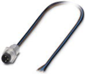
Sensor/actuator panel-mount connector, 3-pos., M8, front/screw mounting with M8 thread, with 0.5 m PVC litz wire, 3 x 0.25 mm 2
