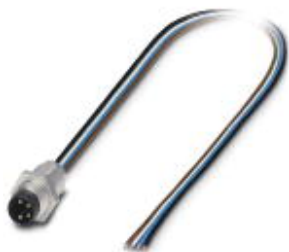
Sensor/actuator panel-mount connector, 4-pos., M8, front/screw mounting with M8 thread, with 0.5 m PVC litz wire, 4 x 0.25 mm 2
