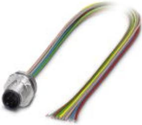
Sensor/Actuator flush-type plug, 8-pos., M12-SPEEDCON, A-coded, front/screw mounting with M16 thread, with 0.5 m TPE litz wire, 8 x 0.25 mm<sup>2</sup>
