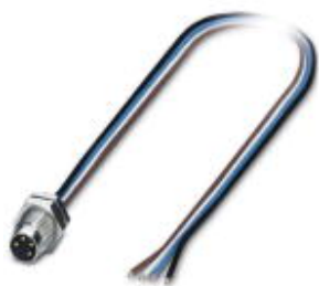
Sensor/actuator panel-mount connector, 4-pos., M8, rear/screw mounting with M8 thread, with 0.5 m PVC litz wire, 4 x 0.25 mm 2
