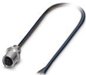
Sensor/actuator flush-type socket, 3-pos., M5, prewall/screw mounting, with M5 thread, with 0.5 m TPE litz wire, 3x0.14 mm 2
