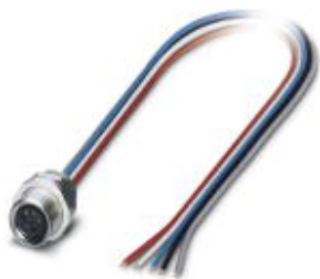
Bus system flush-type connector, socket, DeviceNet, 5-pos., M8, front/screw mounting with M10 fastening thread, with 0.5 m TPE litz wire, 5 x 0.25 mm²
