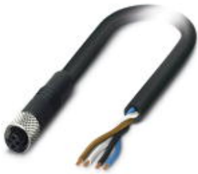
Sensor/Actuator cable, 4-position, PUR, black RAL 9005, free cable end, on Socket straight M5, A-coded, Cable length: 3 m
