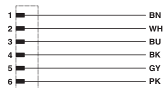
Contact assignment of the M8 plug
