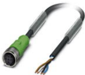
Sensor/Actuator cable, 4-position, PUR halogen-free, black-gray RAL 7021, free cable end, on Socket straight M12, A-coded, Cable length: 1.5 m
