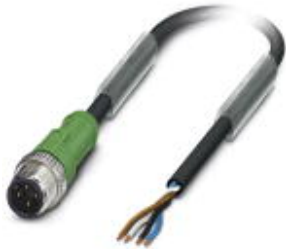
Sensor/Actuator cable, 4-position, PUR halogen-free, black-gray RAL 7021, Plug straight M12, A-coded, on free cable end, Cable length: 5 m
